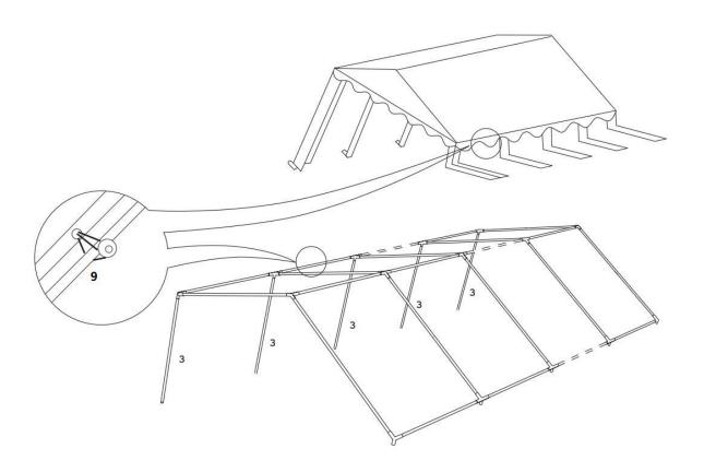
**Step 3.** Attach the legs on the other side. Make sure, that the leg pipes are in vertical position, to avoid overtention
